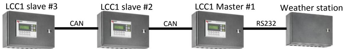
When running cables between the units as shown above, you should remember to place termination at either end of the CAN communication. This is done by means of the SDV003 PCB jumper JP1.
