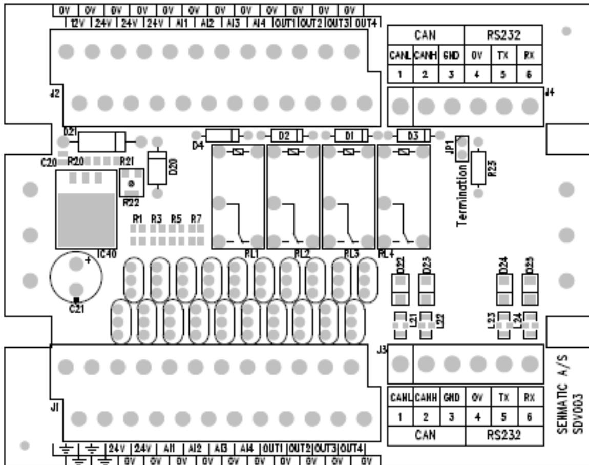
All external connections are connected to connector J1 & J3.
