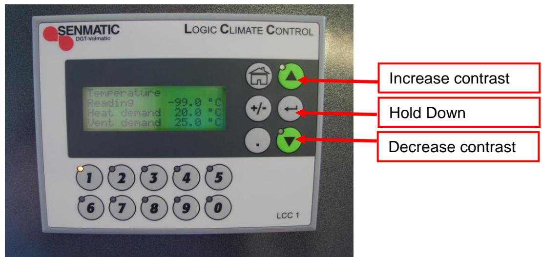
To adjust the contrast press and hold the "Hold Down" button simultaneously with you press on respectively the increase/decrease contrast button.
