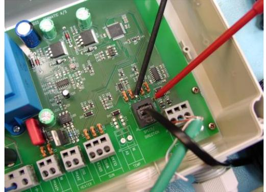
If you put the connector from the weather station in the socket and measure with a multimeter on the connector, you can measure the ohm value from the direction sensor.
