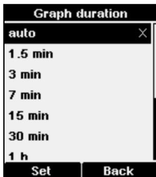
In the **Graph duration** screen, you can select the timescale of the Graph view. The shortest selectable timescale is 1.5 minutes, the longest 32 hours.
