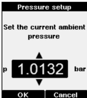
In the **Pressure setup** screen, you can set the current ambient pressure. The pressure information is used when calculating certain humidity parameters, such as mixing ratio (symbol  $x$ ).
