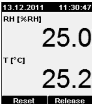
When the screen is held, the top of the display displays the current date and time. This is useful when you want to record the current data (take a photograph or write it down).
