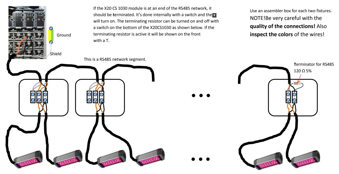
It's possible to make two segments. Each segment connected to one of the two X20 CS 1030 modules.
