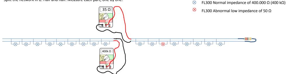
These measurements tells us that we have a lamp with very low impedance to the right.
