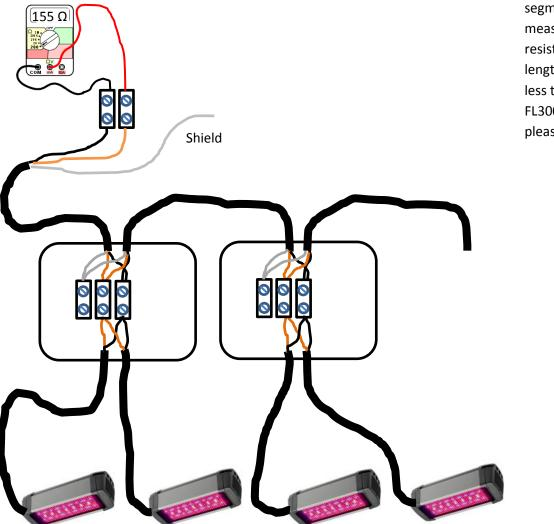
When finished the installation of a network segment, it's important to make an impedance measurement. The impedance is  $120 \Omega$  + cable resistance. The measurement depends on cable length and should be approximately  $150 \Omega$ . <u>Never</u> less than  $120 \Omega$ . Make this measurement with the FL300 powerless. If you see too low impedance, please follow the instructions at the next page.
