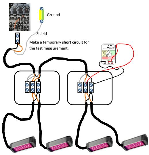
After the installation of 2 assembler boxes, it's time to make a measurement of the cable resistance. Make this measurement with the FL300 powerless.
